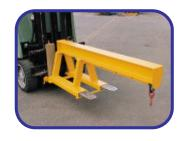
lifting and conveying loads which are not suitable for, or do not require palletising. Supplied with a hook & shackle which can be placed at any of the given load centres.
