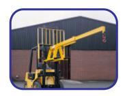
with a conventional jib. The greater length allows previously in-accessible loads to be handled. Manual Extension.
