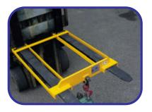
Our Fork Mounted Hooks are a simple and cost effective means of converting the fork lift truck into a mobile crane. Anchor bars at the back of the attachment lock behind the heels of the forks to prevent movement of the attachment.
